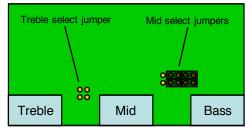
Switch UP = HIGH mid Switch DOWN = LOW mid Treble is fixed high
