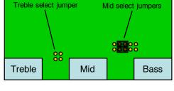
Switch UP = HIGH mid Switch DOWN = MEDIUM mid Treble is fixed high
