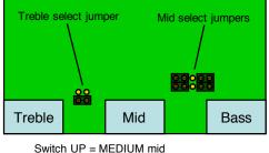
Switch UP = MEDIUM mid Switch DOWN = LOW mid Treble is fixed low
