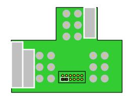
With jumper installed side to side, bass frequency stays at the LOW setting regardless of the switch position.
