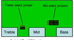
Switch UP = HIGH mid Switch DOWN = LOW mid Treble is fixed low
