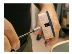
4. Now thread the Truss Rod Remover onto the threaded portion at the top of the Truss Rod. You only need to thread the tool 2-3 complete turns.
