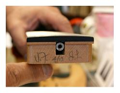
Take extra care when adjusting the Truss Rod. Do not damage the sides of the Truss Rod Channel when making your adjustments.
