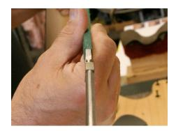
7. Once flipped, reinsert the Truss Rod...
