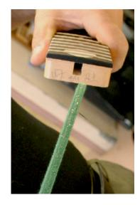
6. Whichever position the Truss Rod was in, flip it over 180 degrees before reinserting it into your bass. In the photos that follow, a Truss Rod that had been in the Normal Position is being flipped to the Reversed Position...
