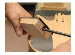
5. Pull the Truss Rod out of the channel in the neck.
