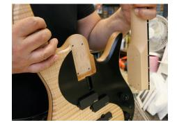
3. Completely loosen the nut using the U-Bend tool that came with your instrument.
