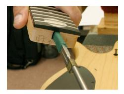
8. Reinstall the Nut and adjust the Truss Rod so that it just begins to come under tension.
