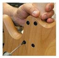
10. You can now string up your bass. Remember to tune your bass <u>before and between</u> making any adjustments after reattaching the neck to the instrument...Allow the bass to settle-in for 24 hours and then make any necessary fine-tuning adjustments.
