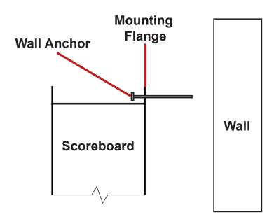
Wall anchors vary based on construction material of the supporting wall. Anchor for mounting supplied by the customer.
