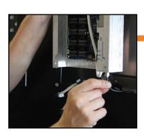
(3.8) At this point you will be able to access a connecting cable at the bottom corner of the driver box that can be unscrewed and allow complete removal of the box. Now your box is ready for maintenance.
