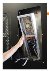
(3.7) To lift driver box out of the cabinet you will need to tilt the top of the box forward and lift up and pull outwards. Now the box is should be removed from the cabinet.
