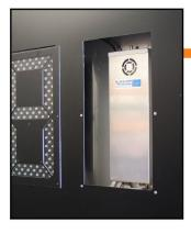
(3.3) With the digit removed you can now see the driver box. The box will look similar to the one pictured. It will also inform you on how many drivers the scoreboard contains. Labeled (Driver: 1 of 1, 1 of 2, or ext.). The cover will need to be removed for the rest of the connection process.
