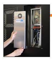
(3.4) To remove Driver box cover, remove the screws and grasp box on the sides. Slide cover down and pull forward to remove.
