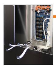
(3.5) Unplug each ribbon cable attached to the driver.
