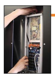
(3.6) At the top of the driver box you can locate a screw that holds the box into place. You can use your hand to untwist this screw to allow removal of the driver box.
