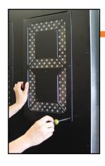
(3.2) Once you have located the driver access digit, remove each screw holding the digit in place. The digit will remain in place once unscrewed and must be lifted out of place. To remove a digit pull the bottom of the digit towards you and then slide top lip of digit down and away from the board.
