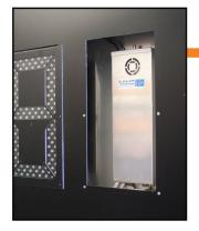
(3.3) With the digit removed you can now see the driver box. The box will look similar to the one pictured. It will also inform you on how many drivers the scoreboard contains. Labeled (Driver: 1 of 1, 1 of 2, or ext.). The cover will need to be removed for the rest of the connection process.
