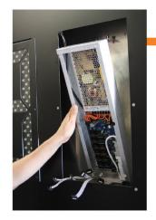
(3.7) To lift driver box out of the cabinet you will need to tilt the top of the box forward and lift up and pull outwards. Now the box is should be removed from the cabinet.
