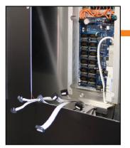
(3.5) Unplug each ribbon cable attached to the driver.
