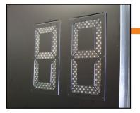
(1.1) You will need to locate the scoreboards driver. The driver can be accessed behind the digit labeled Driver Access. Some scoreboards may have multiple drivers depending on the size of the board and the number of digits.
