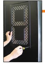
(3.2) Once you have located the driver access digit, remove each screw holding the digit in place. The digit will remain in place once unscrewed and must be lifted out of place. To remove a digit pull the bottom of the digit towards you and then slide top lip of digit down and away from the board.
