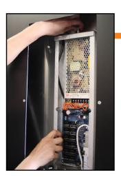
(3.6) At the top of the driver box you can locate a screw that holds the box into place.You can use your hand to untwist this screw to allow removal of the driver box.
