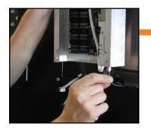
(3.8) At this point you will be able to access a connecting cable at the bottom corner of the driver box that can be unscrewed and allow complete removal of the box. Now your box is ready for maintenance.
