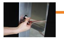
(1.6) On cabinet 1 you will see an opening that will allow you to pass wires through from Cabinet 2 to Cabinet 1 containing the driver box.
