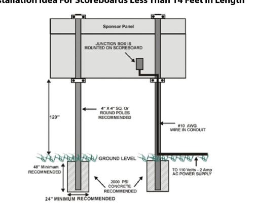
Installation Idea For Scoreboards Less Than 14 Feet in Length
