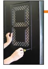
(1.2) Once you have located the driver access digit, remove each screw holding the digit in place. The digit will remain in place once unscrewed and must be lifted out of place. To remove a digit pull the bottom of the digit towards you and then slide top lip of digit down and away from the board.
