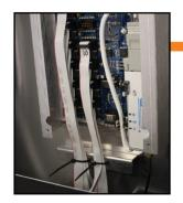
(1.9) Here you can see an example of properly installed and secured cables. Make sure your cables are properly secured. Once you have cables secured replace the driver box cover. This completes the connection of digit cables to the driver box.
