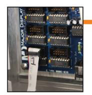
(1.7) The driver panel will have numbers listed on the left side of each plug so that you can simply plug each digits numbered ribbon cable into its corresponding numeral position.
