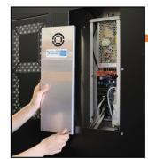
(1.4) To remove Driver box cover, remove the screws and grasp box on the sides. Slide cover down and pull forward to remove.
