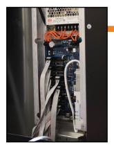
(1.8) Once all ribbon cables for each digit are plugged into the correct place you will need to secure the cables. Do this by grouping each row of cables together in a stacked group. You will find an area at the bottom of the driver box to thread a zip tie through and secure the cables into place.
