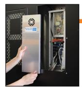
(3.4) To remove Driver box cover, remove the screws and grasp box on the sides. Slide cover down and pull forward to remove.
