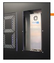
(1.3) With the digit removed you can now see the driver box. The box will look similar to the one pictured. It will also inform you on how many drivers the scoreboard contains. Labeled (Driver: 1 of 1, 1 of 2, or ext.). The cover will need to be removed for the rest of the connection process.
