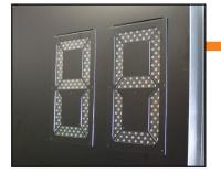
(3.1) You will need to locate the scoreboards driver. The driver can be accessed behind the digit labeled Driver Access. Some scoreboards may have multiple drivers depending on the size of the board and the number of digits.
