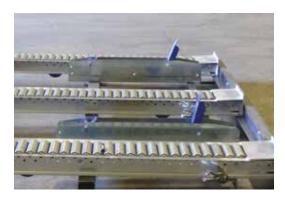
Mallard's Forklift Separator is an automatic pallet release that engages as the front pallet is extracted by the forklift, allowing the rear pallets to gently index forward and again lock into place. Isolating the front pallet and removing rear pallet forces is even more critical at higher elevations where forklift mast capacity is reduced.
