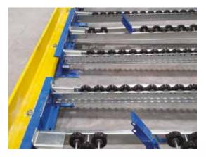
Layer picking uses specialized material handling equipment to select multiple cases, or the entire carton layer, at one time, thus increasing pick rates reducing manual labor costs. Mallard's LP-400 Pallet Separator is used within the layer pick pallet flow system to separate the front pallet until all cases are selected, allowing safe manual removal of the empty pallet.
